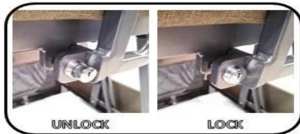
Move the guardrail to the left in order to block it inside the manual safety lock
